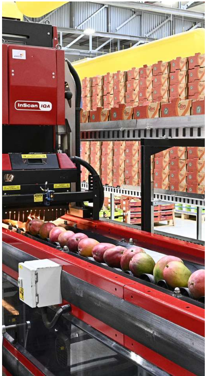
Mango maturity grading on the Aweta machine - SIIM, Rungis, France
